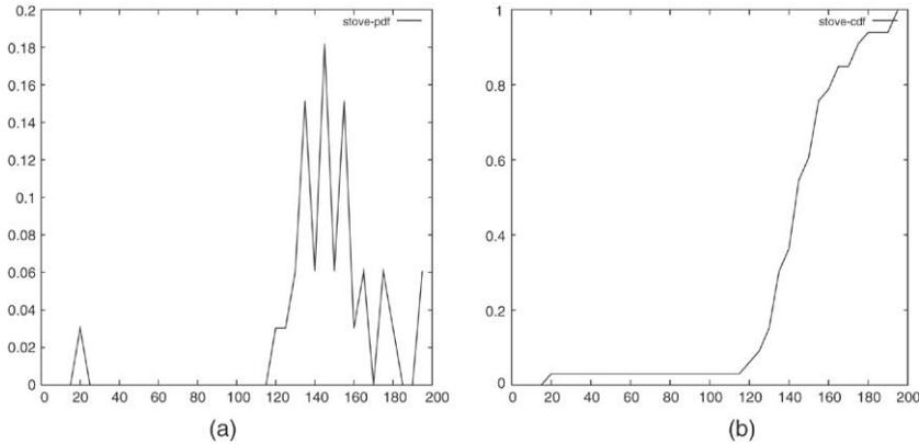
Fig. 3. The probability density function,  $p_{\text{SID}}^{\text{STOVE}}$ , and cumulative distribution function  $P_{\text{SID}}^{\text{STOVE}}$  for the stove (time in seconds).
