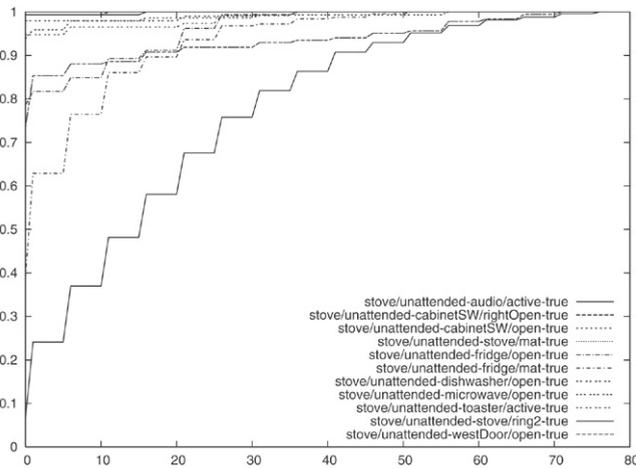
Fig. 4. The cumulative distribution functions for other devices ( $P_{\text{IID}}^{\text{STOVE},d_j}$ ) while the stove is in a hazardous state (time in seconds).
