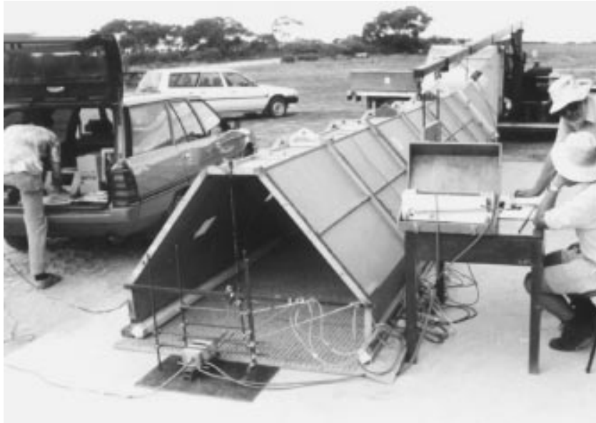
Figure 3. Turbulence probe trials with the AWA wind-tunnel over a 'peg-board' surface.
