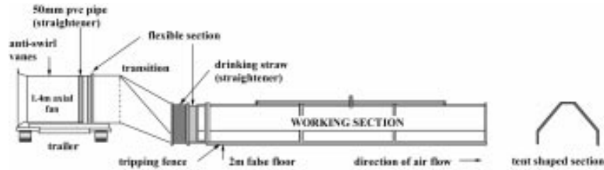
Figure 4. AWA wind-tunnel with a tent shaped cross-section. The working section following the false floor is 5.1 m long by 1.5 m wide by 1050 mm high.
